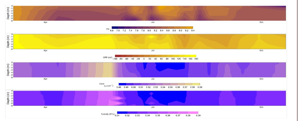
Fig. 4 - Sample results of the General Lake Model from Marion dam. From top to bottom: pH, ORP (mV), Cond. (µ s cm<sup>-1</sup>), Turbidity (NTU).
