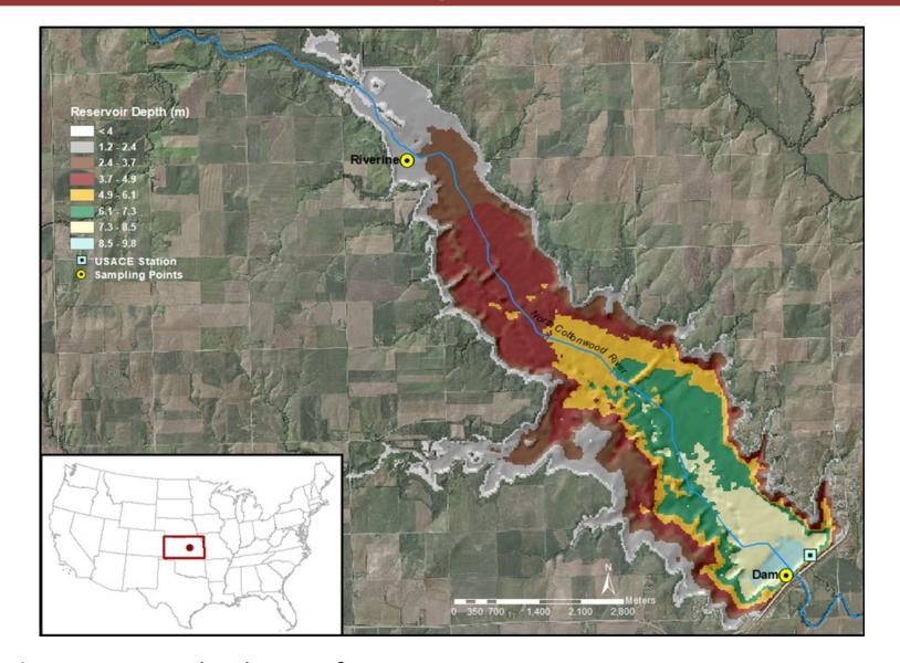
Fig. 1 - Depth chart of Marion Reservoir, Marion County, KS. Marion is a relatively-shallow lake, with a mean depth of 10 feet and a maximum depth of around 30 feet.
